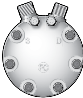
Type FG Vertical O-Ring \frac{3}{4} " x \frac{7}{8} "
